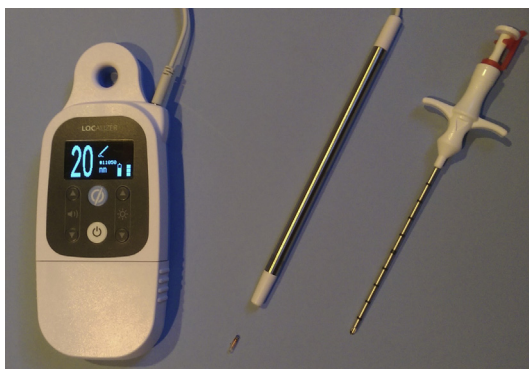
Fig. 3. Non-wire systems have 3 components: a single-use sterilized device preloaded in a needle introducer, a reusable console, and a dedicated handheld intraoperative probe. (Courtesy of Health Beacons, Inc, Concord, MA; with permission.)
